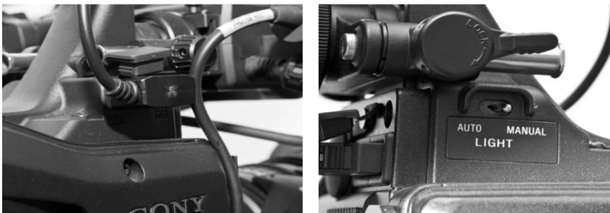
4. To synchronize the light and the ENG camera's Cue/Cut button, turn the light on, and set the ENG camera to Auto mode. Then set the light to the Auto mode pressing the light's Power switch for 3 seconds. To switch to
