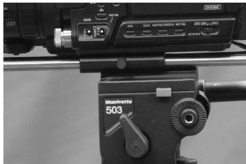
⚠ CAUTION: It is possible to damage the attachment points on the camera as well as the adapter when excessive load is placed on the slide. To reduce this risk always adjust the slide as short as possible.
