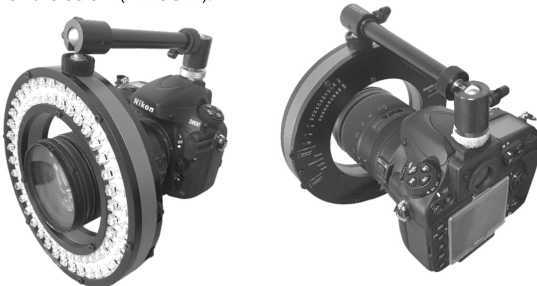
3. Use the ML-PT1 power cable to connect the light to the 12V DC output on the camera, or use Power Tap Connector (ML-PT3) to connect the light to the battery pack or 12V DC output port in V Mount Adaptor. Please ensure the polarity of the power cable is correct. When the polarity is switched, the light might not come on, or it causes malfunction.
