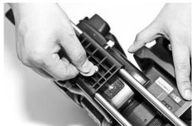
3. Insert the L-bracket slide (ML-SL30 or ML-SL15) into the hole of the Tripod Adapter and tighten the fastening screw. Hook the battery on to the slide and connect it to the light with the power cable (ML-PC1).
