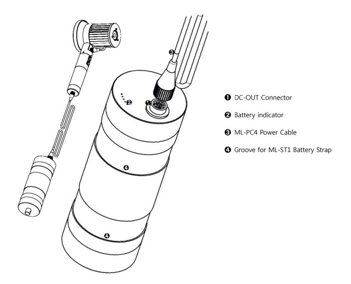
\* ML-BA48W Battery with ML-ST1 Battery Strap
