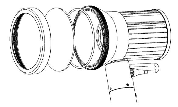
▲ CAUTION: Silicon O-ring must be in the right place with silicon grease for waterproofing. In case the O-ring is damaged or missing, a new O-Ring is required for perfect waterproofing.
