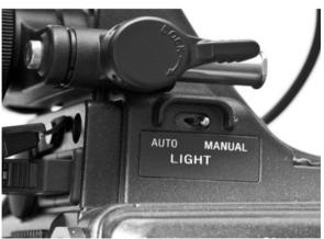
4. To synchronize the light and the ENG camera's Cue/Cut button, turn the light on, and set the ENG camera to Auto mode. Then set the light to the Auto mode pressing the light's Power switch for 3 seconds. To switch to
