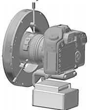
2. To use the supplied battery, fasten the battery to the camera using the Tripod Adapter (ML-AT1) and the L-Type(ML-SL30) or C Type(ML-SL10) Slide. Start by installing the Tripod Adapter (ML-AT1) to the camera using the screw at the bottom of the adapter.
